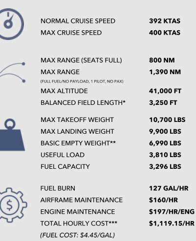
\*Consideration must also be given to, but not limited to: passenger weights, baggage weight, winds, runway length, temperature and airport elevation.
